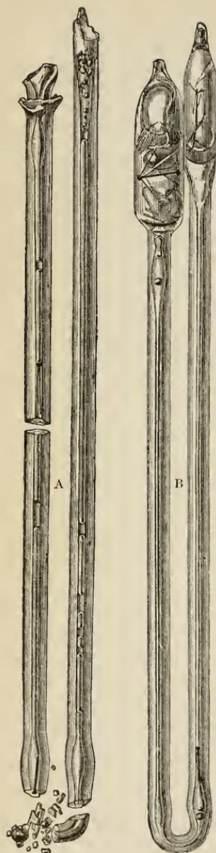
FIG. 70.—Thermometer tubes broken by pressure at Station XXV. A, Thermometer No. 39; B, No. 42.
