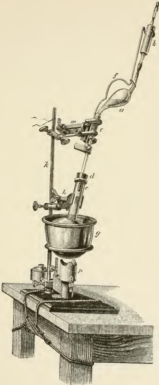
FIG. 3.—Apparatus for collecting the Atmospheric Gases from Sea-water.
